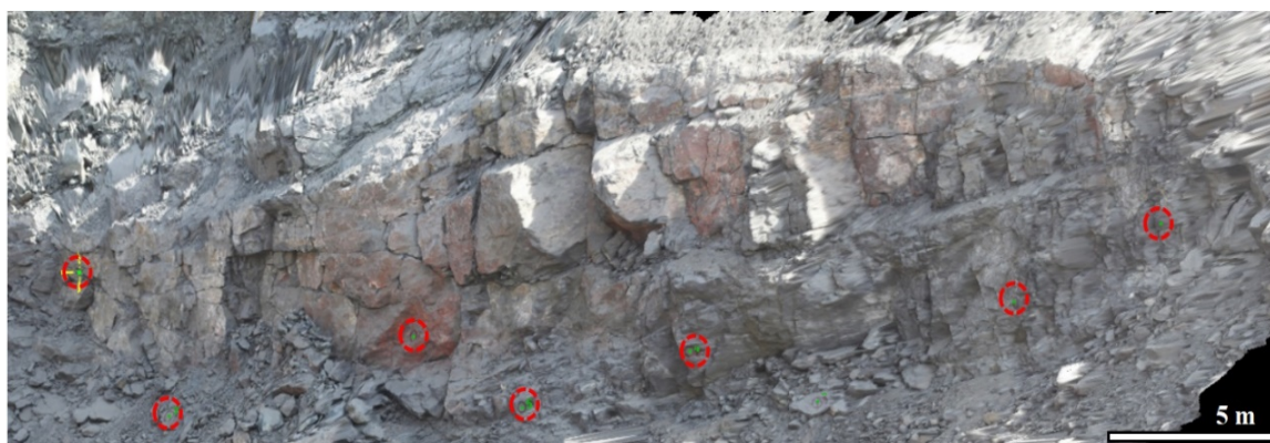
Figure 1. Generated 3D image of bench face (location of control points is shown by red circles).
