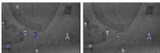
Figure 11. Center detection of ROIs with possibility of presence of one pedestrian (a), several pedestrians (b).
