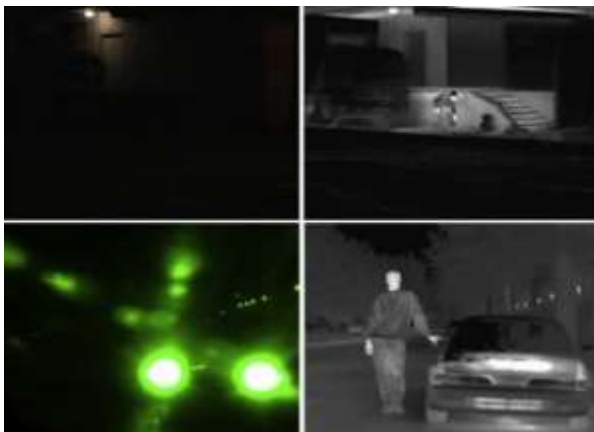
Figure 1. Visible images (left column) and thermal images (right column) of the same scenes that pedestrians are detected in thermal images with insufficient or over illumination [4].
