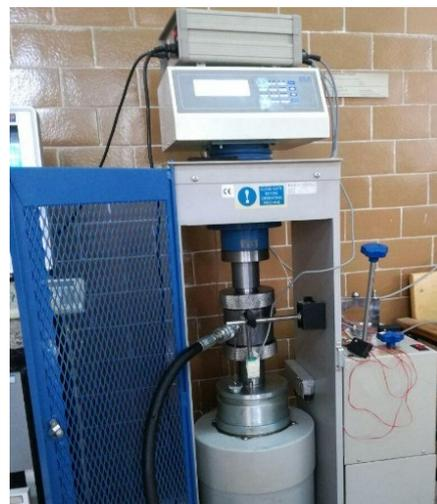
Figure 8. Testing specimens by triaxial cell.
