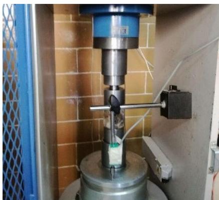
**Figure 9. Loading on specimen in the absence of confining pressure.**
