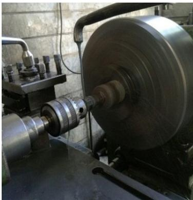
Figure 5. Creating notches on the base of sandstone specimens.
