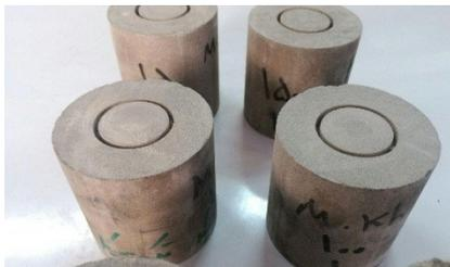
Figure 6. Prepared sandstone specimens.
