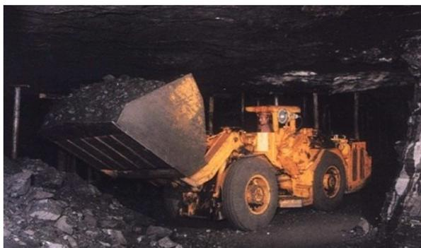
**Figure 2. A typical LHD vehicle performing a loading operation.**
