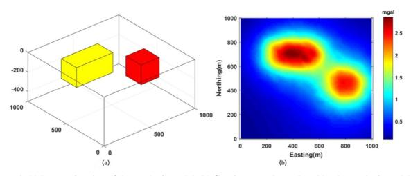
Figure 1. (a) Perspective view of the synthetic model. (b) Gravity anomaly produced by the synthetic model with 3% Gaussian noise.
