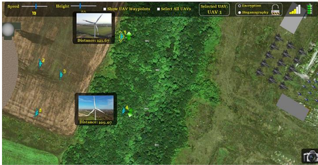
Fig. 3. Two simultaneously occurring collisions and their accordant temporal in-place UAV camera displays at the back of the UAV icons.
