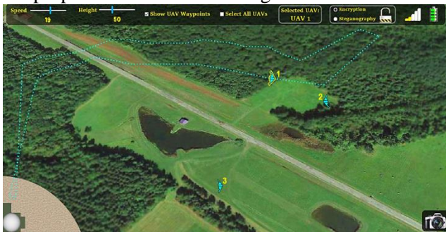
Figure 2. Overall view of the proposed IAI for three UAVs. The selected UAV has been highlighted in yellow and the waypoints of UAV No. 1 have been displayed in cyan.
