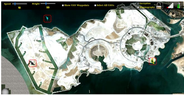
Figure 6. Different luminance of the UAVs' icons that inferred by fuzzy inference based on their local background luminance. Each one of the UAV icons has been highlighted in dashed red square.
