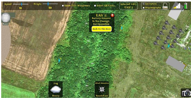
Fig. 4. Temporal in-place user guideline window that has been displayed when a given UAV (UAV No. 1) has not been able to continue its operation.
