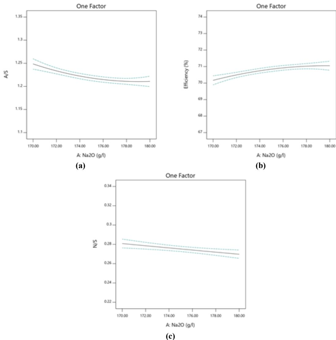
Figure 2. Effect of Na<sub>2</sub>O on a) A/S, b) N/S, and c) digestion efficiency at a constant temperature, lime, and residence time.
