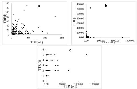
Figure 2. a) Serial-correlation test of group loader 1 (TBF), b) serial-correlation test of group loader 1 (TTR), c) serial-correlation test of group dump trucks 2, 3, 4, 5, 8 (TTR).
