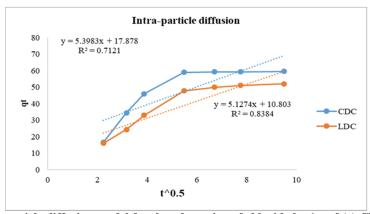
Figure 10. Intra-particle diffusion model for the adsorption of chloride by 1 g of (a) CDC and (b) LDC; conditions: initial chloride concentration: 100z0 mg/L, speed stirrer: 500 rpm, temperature: 298 K.
