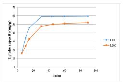
Figure 5. Relationship between the chloride uptake capacity by CDC and LDC and the time ( $C_0 = 1000$  mg/L, T = 25 °C, adsorbent amount = 1 g).
