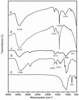
Figure 3. FT-IR spectra for (a) diatomite, (b) chitosan, (c) CDC, (d) MgAl-LDH, and (e) LDC.
