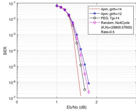
FIGURE 1. The constructed APM codes with different girths against Random and PEG LDPC codes
