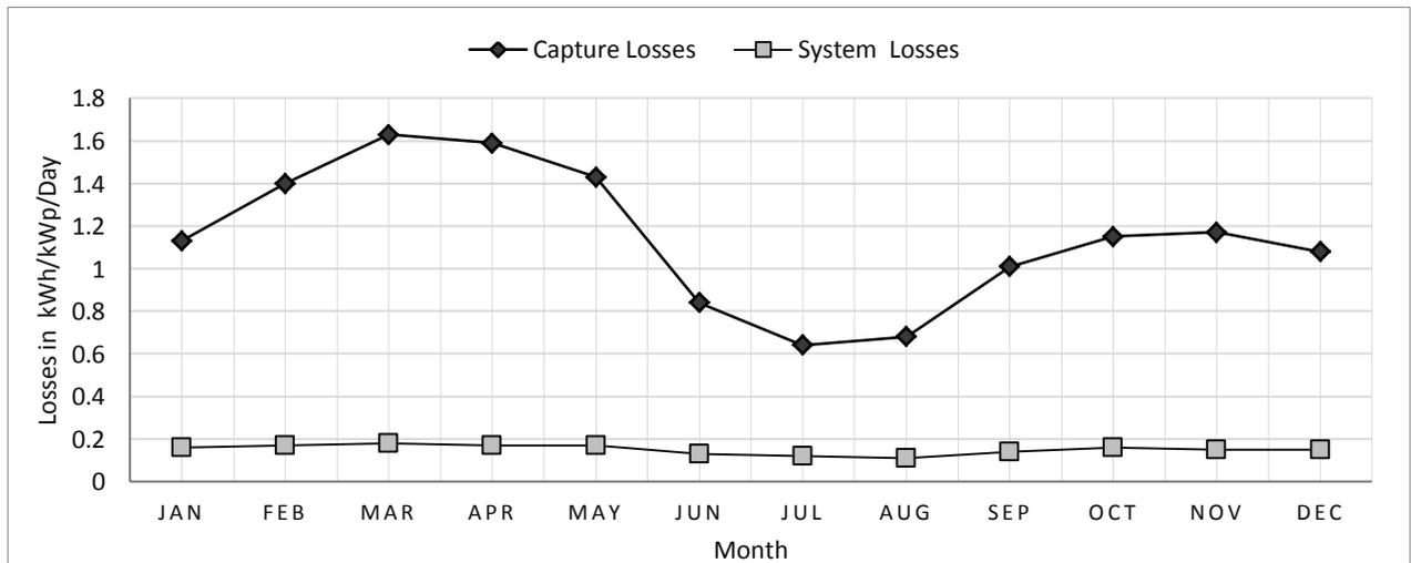
Figure 5. Comparison of capture and system losses for case 2.
