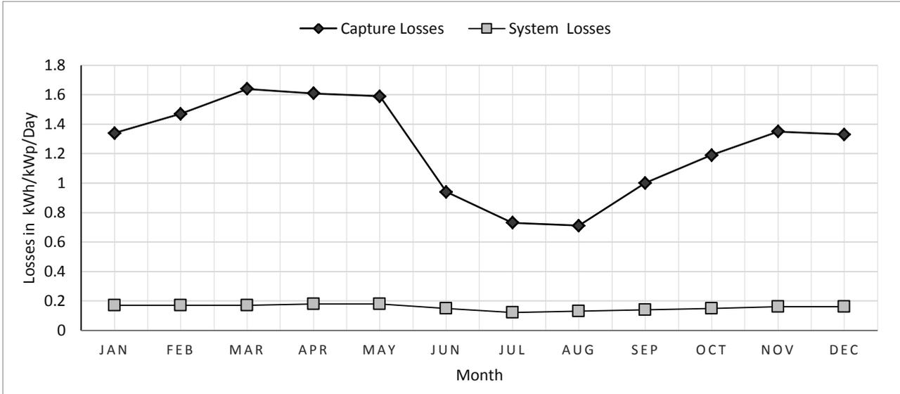
Figure 3. Comparison of capture and system losses for case 1.
