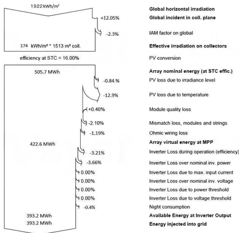
Figure 2. Loss diagram for case 1.
