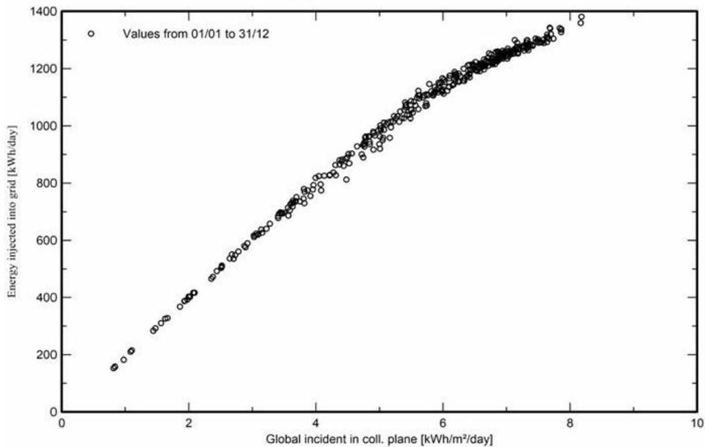
Figure 6. Daily input/output diagram for fixed angle.
