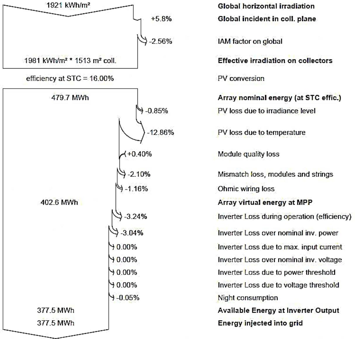
Figure 4. Detail losses diagram for case 2.
