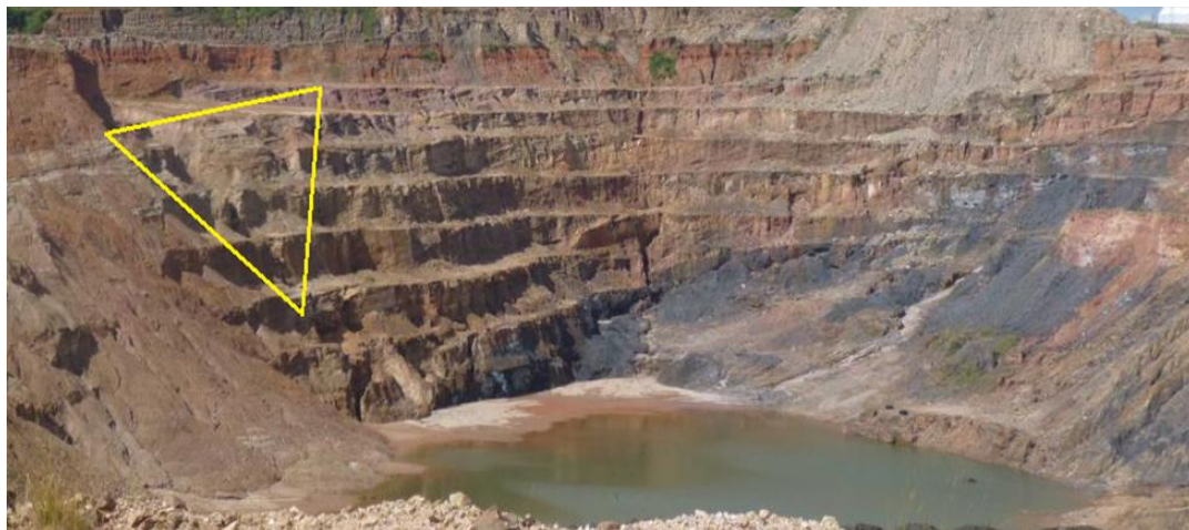
Figure 2. Wedge failure induced by presence of ground water at (COP F&D).
