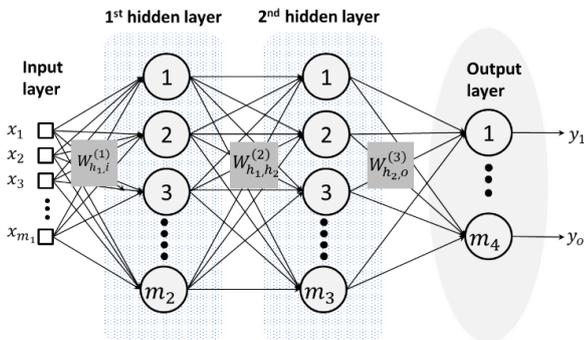
Figure 4. Structure of multi-layer perceptron.
