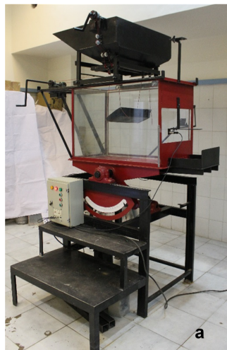
Figure 2. Tilting table machine a) picture, b) schematic diagram [26].
