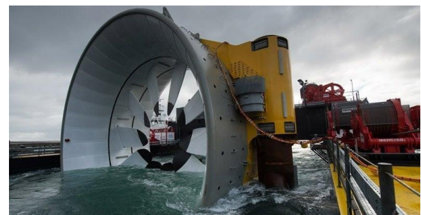
Figure 12. Tidal stream generator [15].
