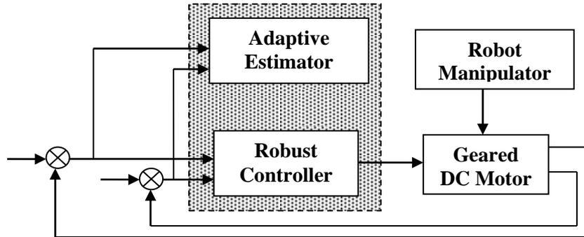
Figure 1. Proposed robust RBF network control.
