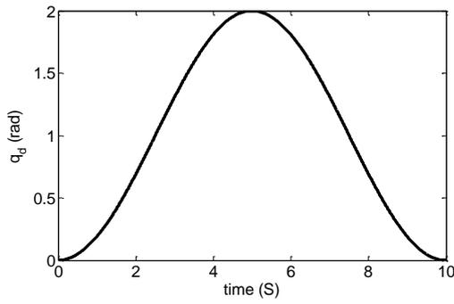
Figure 2. The desired joint trajectory.
