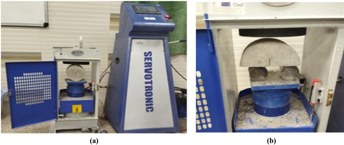
Figure 2. Experimental set up for a) NBD test and b) SCB test.
