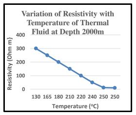
Figure 2. Variation of resistivity with temperature of thermal fluid at Puga (depth, 2000 m).
