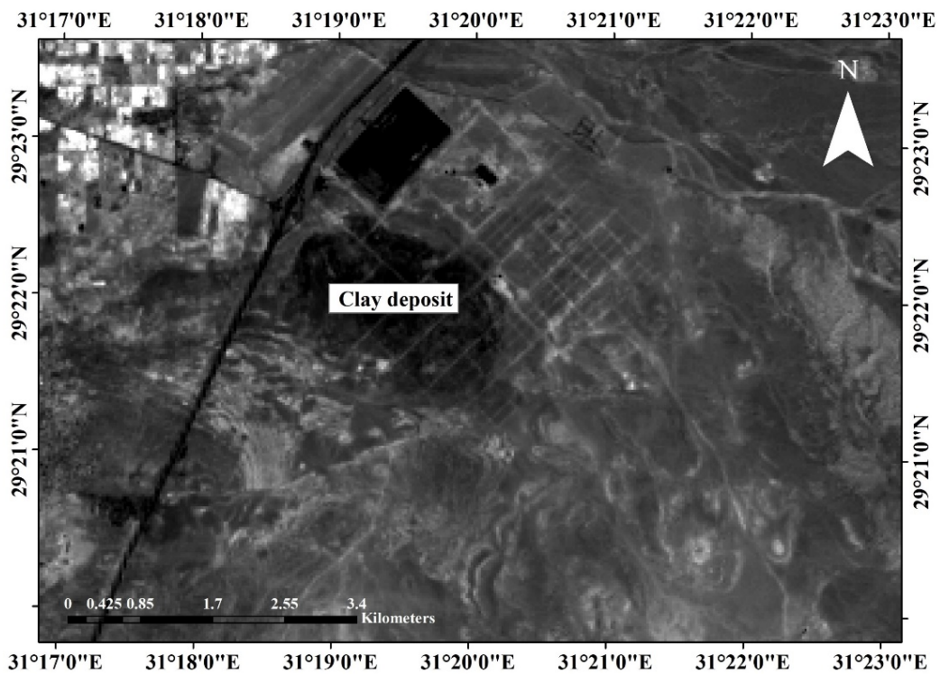
Figure 10. Band 6/band 7 ratio image in grayscale that discriminate clay layer of Pliocene deposit.
