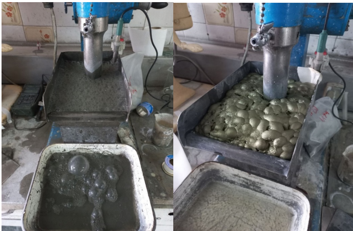
Figure 1. Sarcheshmeh flotation test using DENVER flotation cell (left) standard flotation; (right) bio-flotation.
