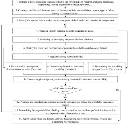
Figure 2. Implementation algorithm of Failure Mode and Effects Analysis [65], [66].
