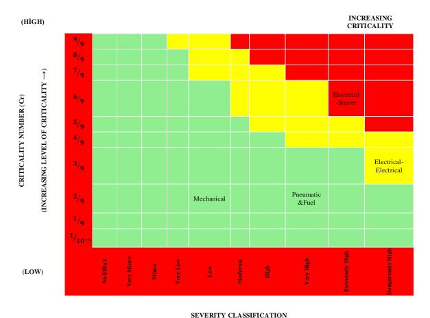
Figure 10. Qualitative criticality matrix for different failure modes (intensity-criticality).
