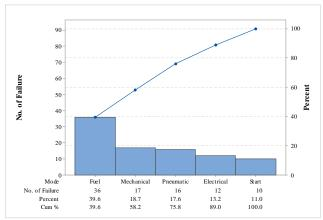
Figure 5. Diagram of dump truck engine breakdown mode.
