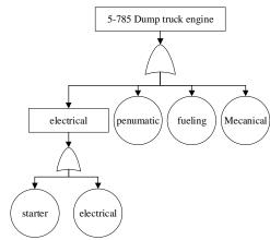
Figure 4. 5-785 Dump truck engine FTA diagram.
