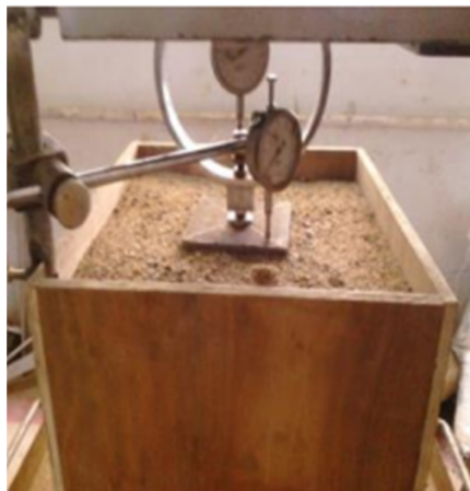
Figure 5. Setup of square footing
