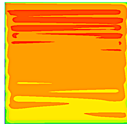
Figure 9. Contours of water content (%) at the interface of cathode catalyst layer and membrane at 0.5 V.
