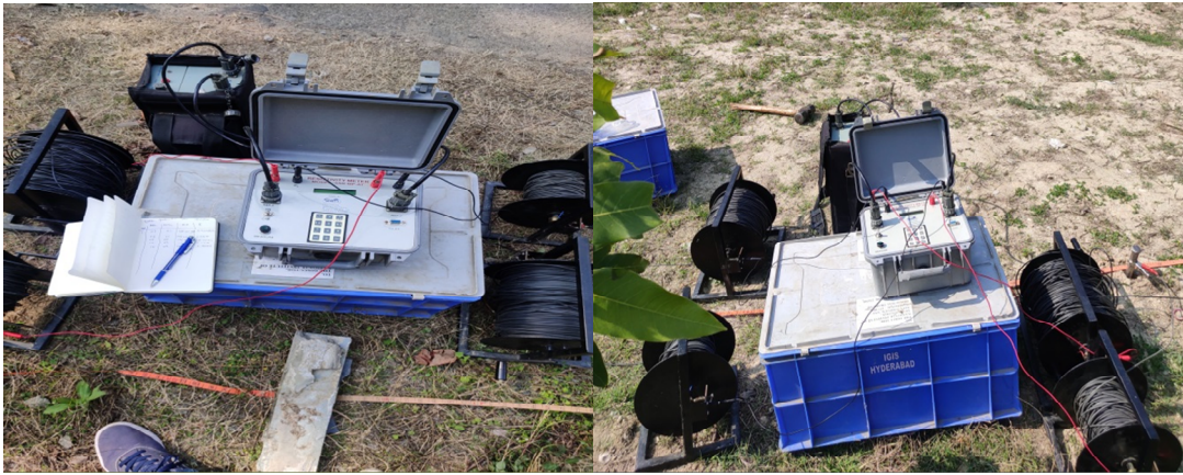
Figure 3. Resistivity meter (Model: SSR-MP-AT).
