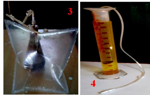
Figure 1. Experimental setup of the anaerobic digestion in this study: 1) inoculums development; 2(A) the arrangement of the anaerobic digestion; 2(B) fermentation processes by circulation of hot water for temperature maintained, 3) produced biogas in the gas bag, 4) barrier solution for the gas measurement through fluid displacement.
