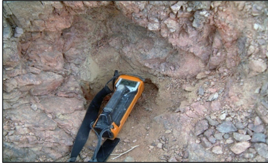
Figure 4. Field in situ measurements of gamma activity by a scintillometer detector (model RS-230).
