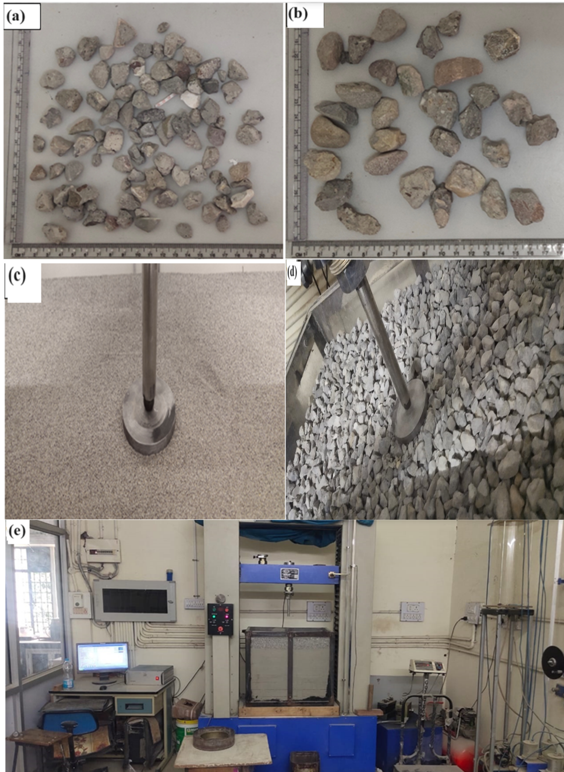
Figure 1 (a) RCW -5 mm; (b) RCW-10.6 mm; (c) Prepared sand test bed, (d) Prepared RCW test bed; (e) Test setup
