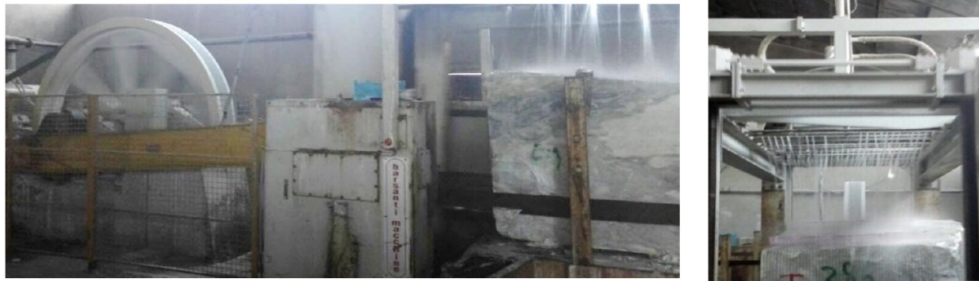
Figure 1. Illustration of the gang saw machine used in this paper [66].
