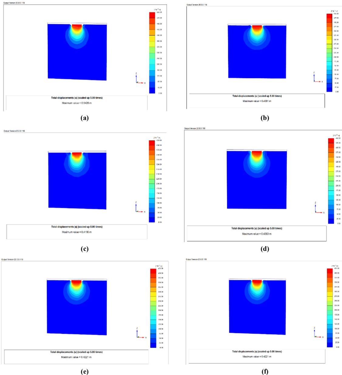
**Figure 6.** The displacement along the cross-section view for soil sample with  $\phi = 34^\circ$  (a) Soil sample without geotextile; (b) Geotextile is provided at 0.2B depth; (c) 0.4B depth; (d) 0.6B depth; (e) 0.8B depth; (f) 1.0B depth.
