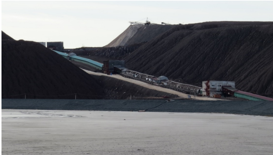
Figure 1. Conveyor line for transportation of halite waste to a salt dump at one of the potash enterprises of the Verkhnekamskoe Potash Deposit, Perm Krai, Russia.
