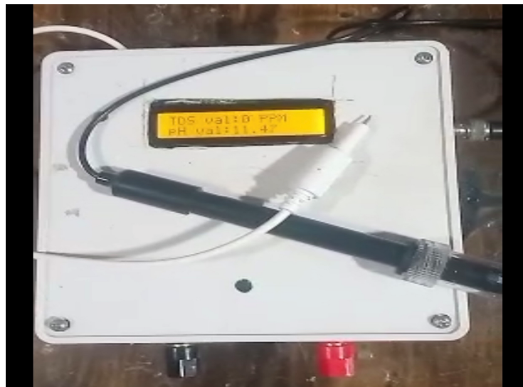
Figure 7. Fully functional Prototype (the red and black nob are provisions for 8watt solar panel).
