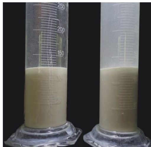
Figure 10. Effect of pulp pH on water turbidity when pulp solid percentage is high, Acidic pH (right), Alkaline pH (left).
