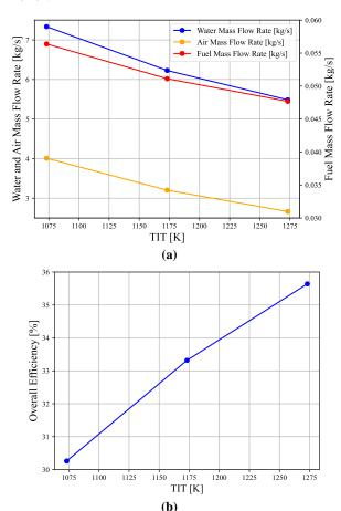
Figure 4. Effect of TIT on a) mass flow rates of the streams and b) overall efficiency.
