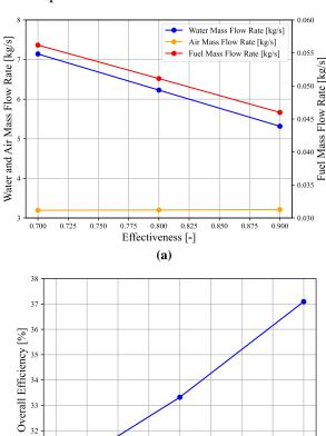
Figure 2. Effect of heat exchanger effectiveness on a) mass flow rates of the streams and b) overall efficiency.
