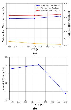
Figure 3. Effect of CPR on a) mass flow rates of the streams and b) overall efficiency.
