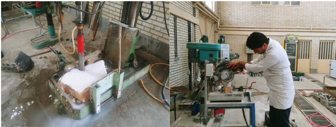
Figure2. Rock coring and preparing in the laboratory
