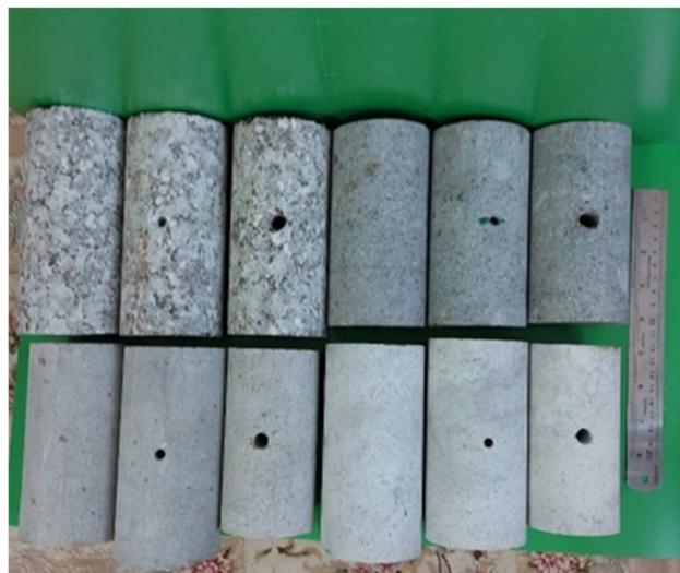
Figure 3. Final specimens prepared from four types of rock with different hole diameters
