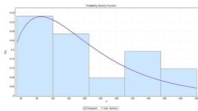
Figure 5. Distribution function of Hyundai excavator repair time 330-2.
