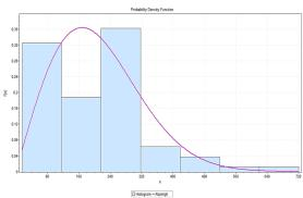
Figure 3. Distribution function for repair time of Komatsu 400 excavator.
