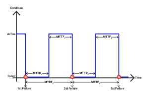
Figure 1. The concept of average repair time and time between failures [13].
