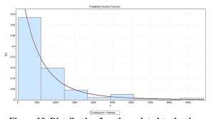
Figure 10. Distribution function related to the time between failures of crusher.
