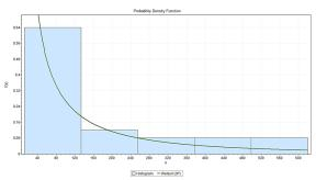
Figure 8. Distribution function of time between failure of Hyundai 330-2 excavator.
