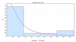
Figure 7. Distribution function of time between failure of Hyundai 330-1 excavator.
