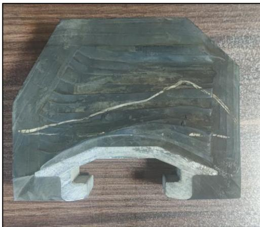
Figure 22. Real profile of the rubber lifters of the Meskavan ball mill.
