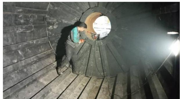
Figure 23. Installation of designed liners and lifters of the Meskavan ball mill.
