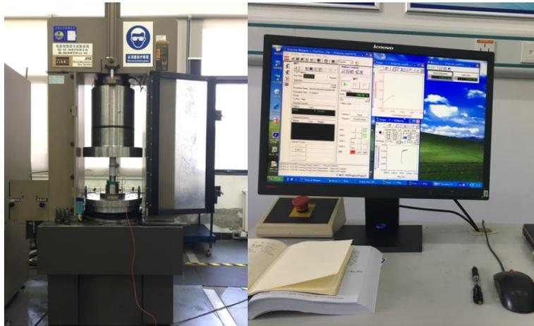
**Figure 3. MTS815.02 Electrohydraulic Servo-controlled Rock Mechanics Testing System.**
