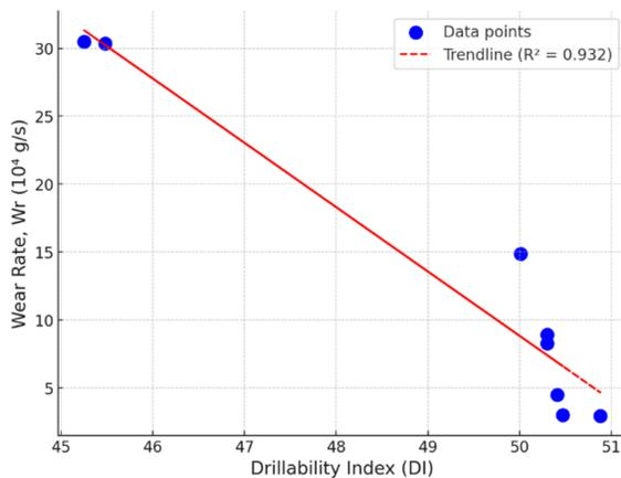
**Figure 5. Wear Rate against Drillability Index for Button Bit**
