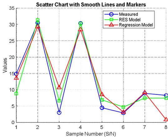
Figure 7. Comparison of RES and Regression Predictions with the Measured Bit Wear
