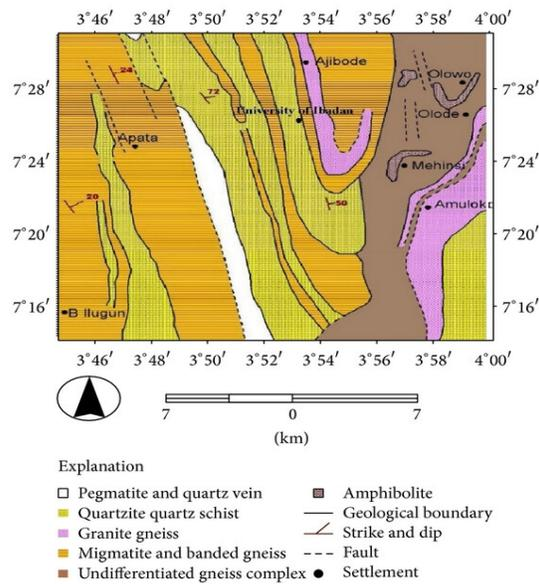
Figure 1. The Geology of Oyo State [51]
