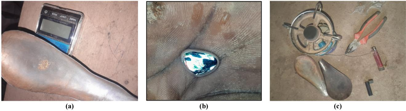
**Figure 8. Ore recovery and sales equipment. a) Electronic balance and metal spoon; b) Mercury; c) Butane gas for drying gold.**
