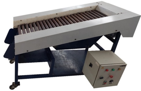
Figure 4. Performing laboratory roller screen tests for classifying green iron ore pellets.
