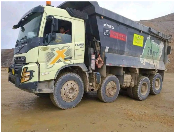
Figure 3. Haul trucks with 26 m 3 capacity used in the mining operations
