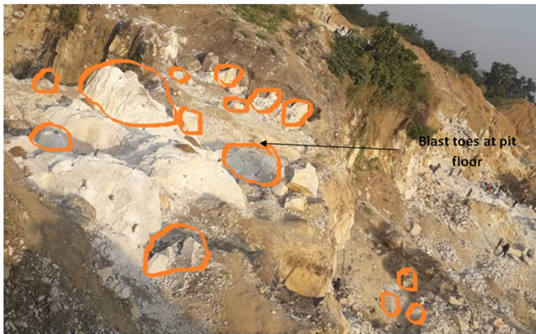
Figure 1. Evidence of toes after loading operation at Fanalou Quarry Pits
