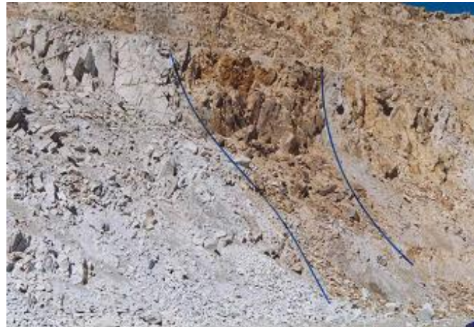
Figure 2. The change in color refers to dyke intrusion in Sungun Porphyry (northern 2300m bench, NW view).
