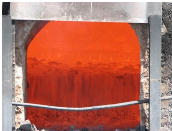
Figure2. Bee-hive oven ready to discharge [13].
