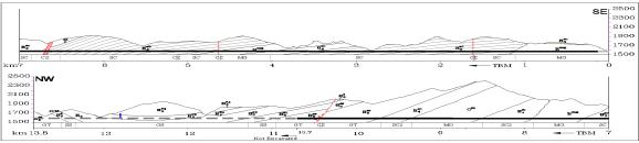
Figure 4. Engineering geological profile of tunnel Lot-2 [28].
